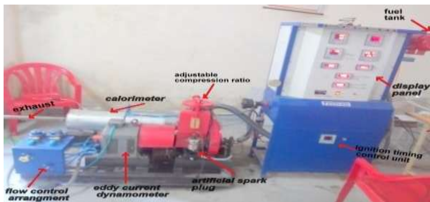
Fig. no.1: Experimental Set-up Of MK -25 HSP Engine
